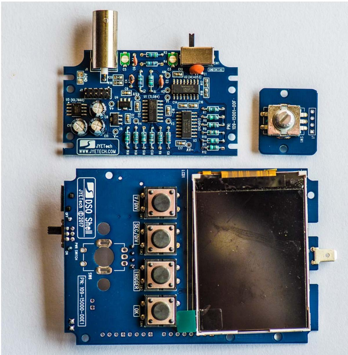
During initial assembly of the Main PCB components, it helps to tape the ‘unattached’ side of the LCD (bottom in the above photo) to the PCB using ordinary adhesive tape, or similar, to stop it flopping around and potentially damaging the thin flex-PCB connections on the other side.
