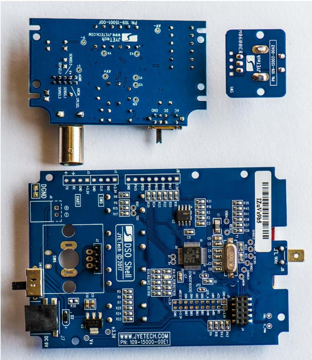
Take special care with the BNC connector (J1) soldering on the Analogue PCB. So it will fit easily through the top-panel hole provided for it, it should be 'square' to the Analogue PCB's edge (i.e. at right angles). Due to the 'slop' in the mounting holes, it is easy to accidentally solder it slightly crookedly.
